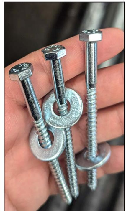
Depending on the type of spa, a piece of wood is placed on the side panels of the spa to protect it in shipping. The wooden supports are installed with several 7/16" (11mm) bolts, once the spa is in its final resting place, remove these with an 11mm socket.
