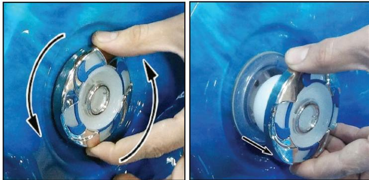
**Note: have the jets turned off when removing jet inserts, it will be easier to remove when there is no water flow through it.**
