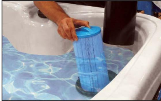
**Note:** Make sure you have removed and soaked the spa filter cartridge in a bucket of water for at least 30 minutes. This will remove air pockets inside of the filter.
